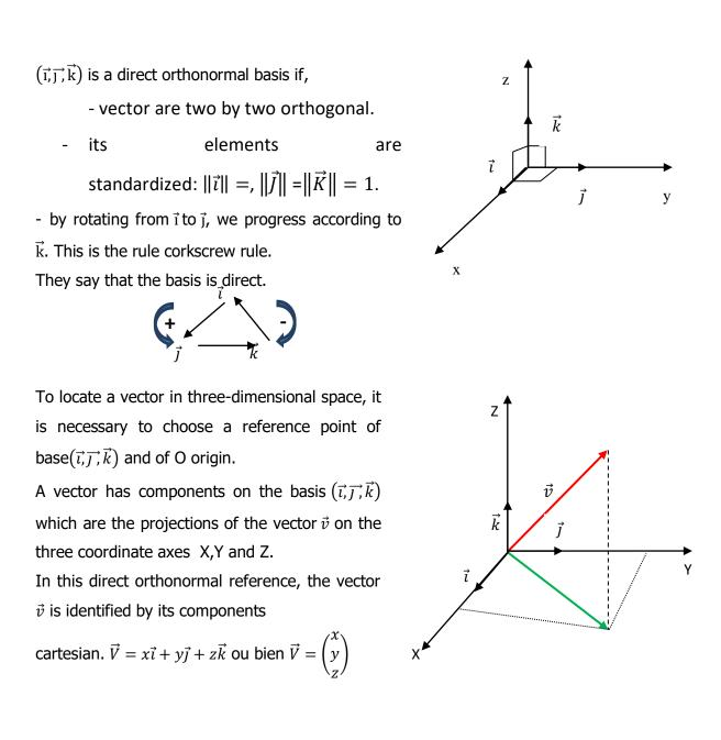
**Modulus of a vector:** The standard modulus of a vector  $\vec{V}$  is represented by  $\|\vec{V}\|$ . In the reference (O,X,Y,Z), equipped with an orthonormal system $(\vec{i},\vec{j},\vec{k})$ , the norm of the vector is given by:  $\|\vec{V}\| = \sqrt{x^2 + y^2 + z^2}$ .
